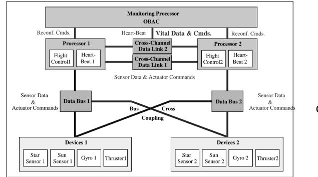
ESA Project DDV validation of the exception handling of a fault-tolerant system
